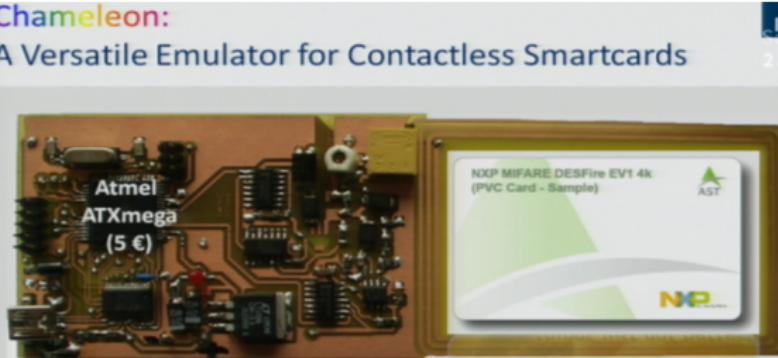
The image shows the Chameleon hardware, which consists of a small printed circuit board (PCB) with various electronic components. An Atmel ATXmega microcontroller is prominently labeled on the board. Next to the hardware is a physical MIFARE DESFire EV1 4k card, which is a standard PVC card with a green and white design, featuring the NXP logo.
